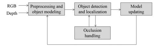
Figure 1. Processing diagram of proposed tracking method.
