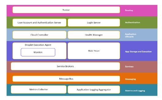
Figure 3. Cloud foundry components
