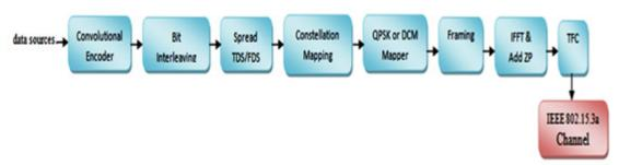
Figure 1: The transmitter architecture for the MB-OFDM system
