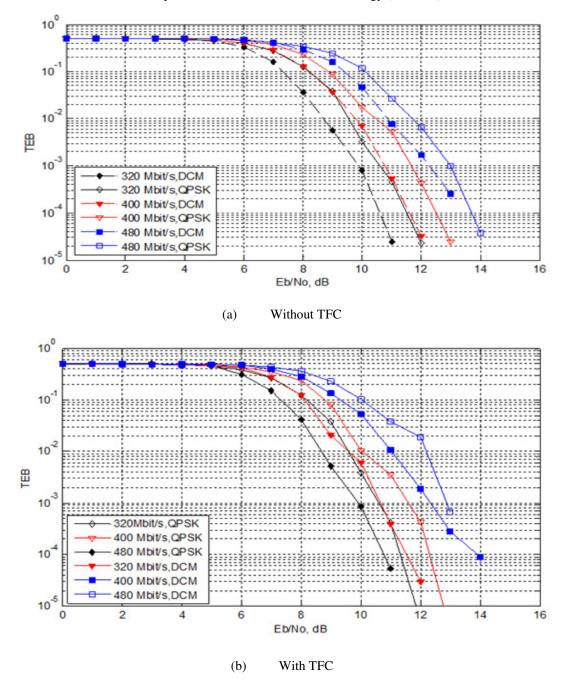
Figure 3: DCM versus QPSK for high data rates of 320 Mb/s, 400 Mb/s and 480 Mb/s Simulation in the case of CM1 (LOS) without TFC n°5 and with TFC n°1.
