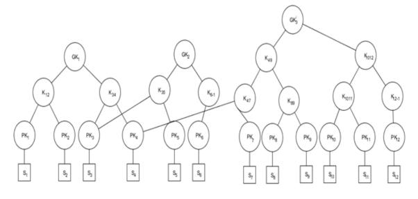
Fig.2 Key Tree after  $s_{12}$  joins  $G_3$ .
