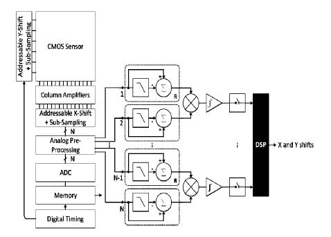
Figure 2: Implementation of NCC algorithm in the new Imaging architecture
