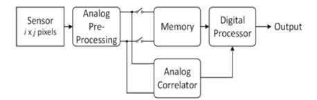
Figure 1: Proposed Architecture for the new Imaging systems
