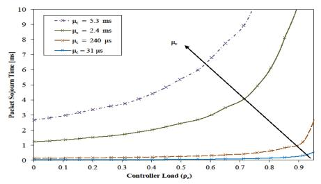
Figure 5: Effect of the controller service rate  $\mu_c$
