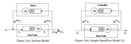
In an OpenFlow network, let  $q_1^{nf}$  be the probability that the packet goes to the controller in case there is no flow entry in flow-table of the node, then in order to use the Jackson network to represent the OF-based SDN we have to adjust  $q_1^{jack}$  by demanding that the input rates to the nodes in both the models are the same. Hence
