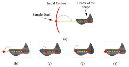
Figure 6.The movement of a pixel on the curve. (a) Initial state. (b) After first step. (c) After secondstep. (d) After third step. (e) After fourth step – Edge found.
