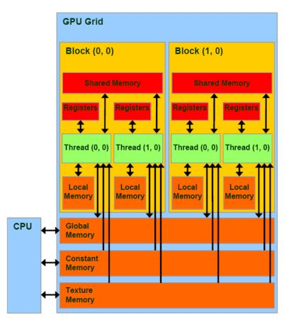
Figure 3.GPU hardware architecture and memory types [20].
