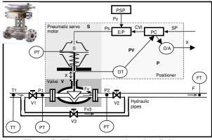
Figure 3. Electro-pneumatic valve Schema.
