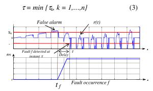
Figure 1. Fault detection by thresholding technique
