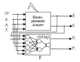
Figure 4. Schema of Neural Networks faulty model NNFM(j).
