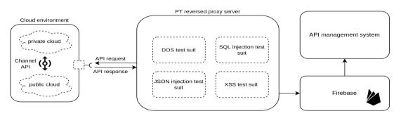
Figure 1. High-level architecture
