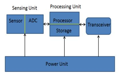
Figure 2. Structure of a sensor node
