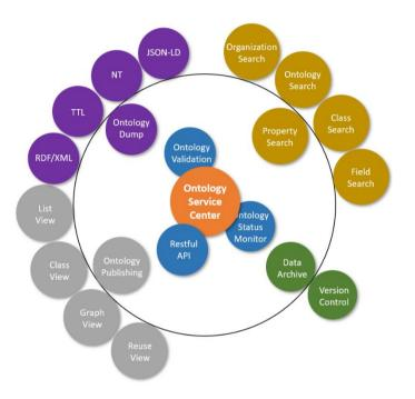
Fig. 3 Functional architecture of Ontology Service Center
