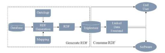
Fig. 2 Process framework of the linked data system
