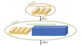
Figure 2. The squeeze and expand Module architecture
